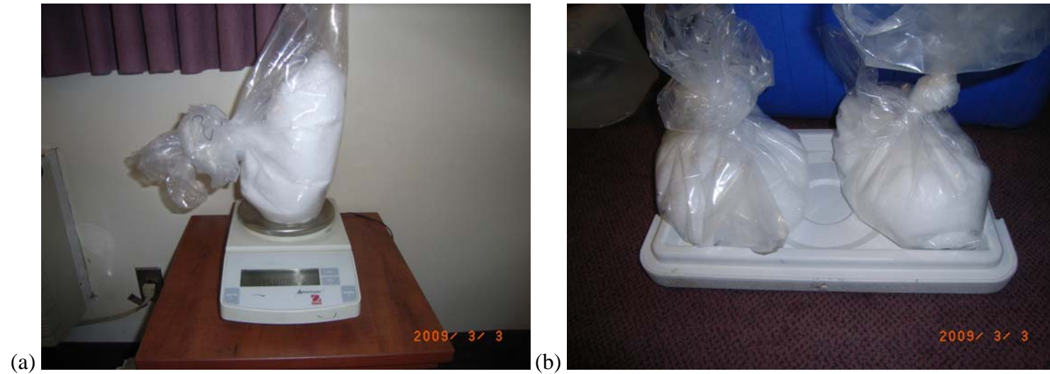
Figure 3. Photographs of the snow processing procedures: (a) measuring the total weight of snow collected, and (b) allowing the samples to thaw at room temperature.
